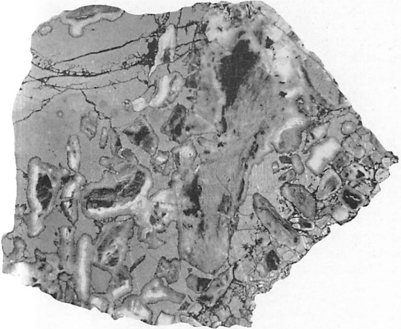
FIG. 1.—Vein breccia. Native arsenic (grey) cementing fragments of carbonated wall-rock (dark grey to black) which are rimmed by colloform dolomite (white to grey). Shrinkage cracks in arsenic in upper left and lower right. Natural size.
