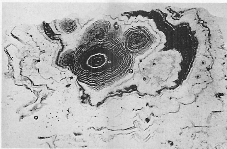
FIG. 6.—Small quartz concretion in anhydrite. Plane light. \times 38 .
