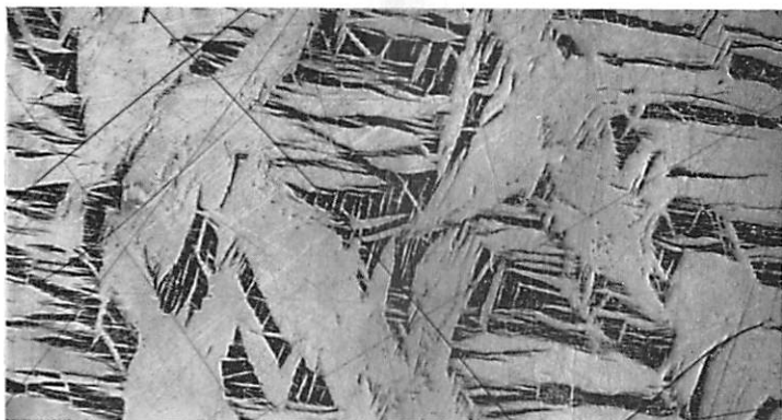
FIG. 16.—Intergrowth of dyscrasite (white) with subordinate antimonial silver (black), Buffalo Mine, Cobalt, Ontario; polished section etched with KCN; vertical illumination ( x -ray powder photograph in Fig. 12); \times 66 .
