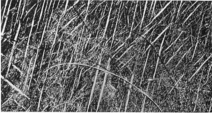
FIG. 15.—Intergrowth of antimonial silver (black) with subordinate dyscrasite (white), Kerr Lake Mine, Cobalt, Ontario; polished section etched with KCN; vertical illumination ( x -ray powder photograph in Fig. 11); \times 66 .
