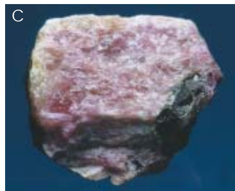
Tenebrescence in sodalite (variety hackmanite) from the Ilímausaaq alkaline intrusion, South Greenland. A. Sodalite in white light (the black mineral on the right is steenstrupine). B. Same specimen viewed with longwave UV light. Colors are similar in shortwave UV. C. Same specimen viewed in white light after being exposed to ultraviolet light for several minutes. In bright light, this purple color will fade to the original yellowish-green .
